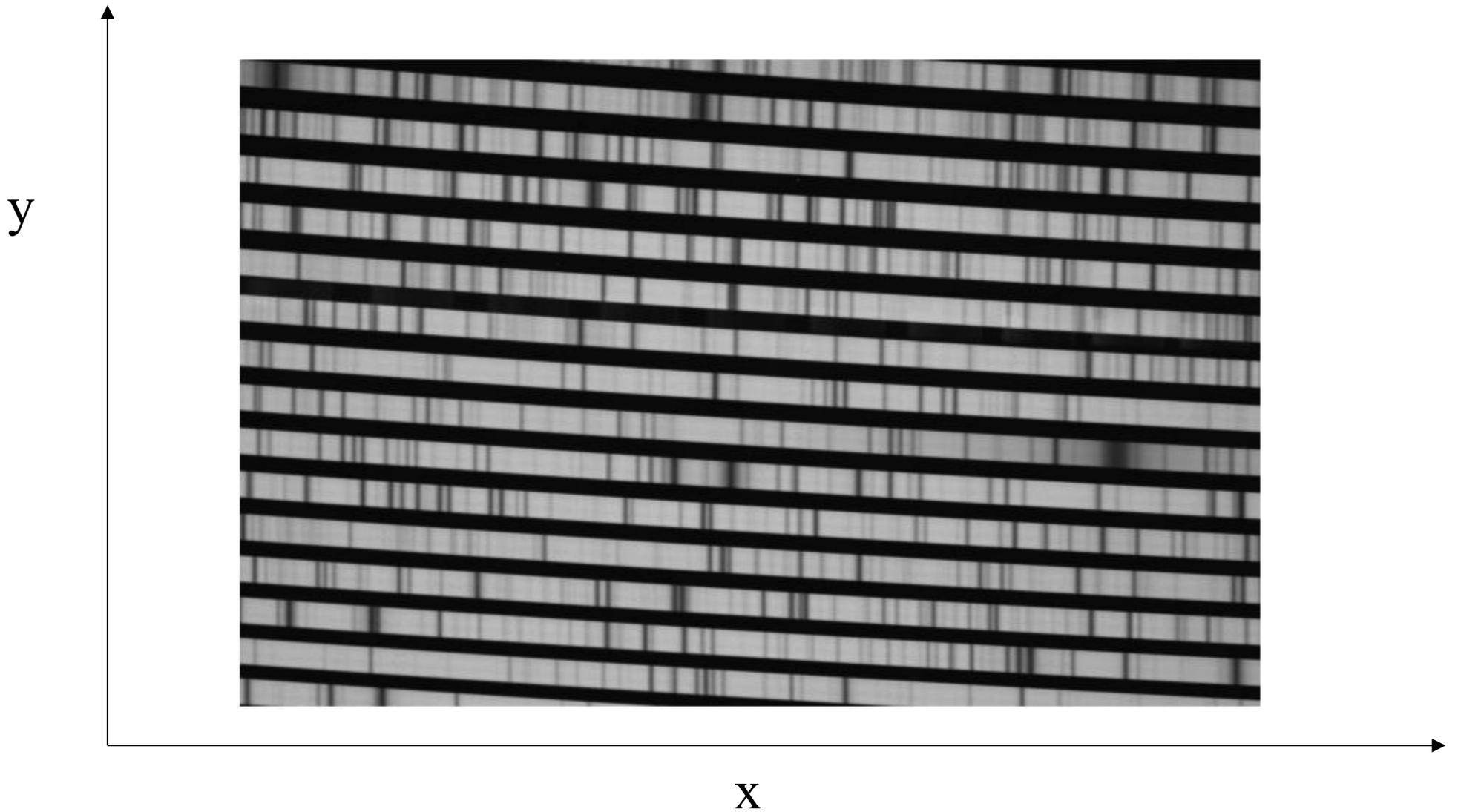
On a detector we only measure x- and y- positions, there is no information about wavelength. For this we need a calibration source
